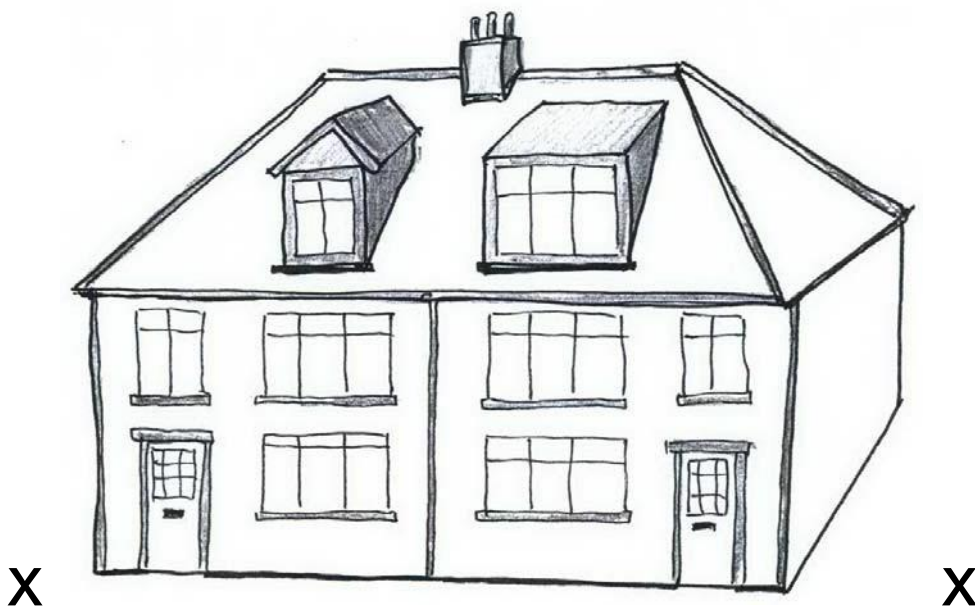
Figure 11 Front dormers on houses
